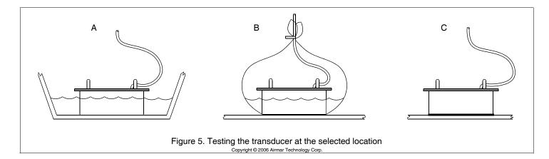
C.**For any location**—If the hull surface is not smooth, grind it with a disc sander. Coat the active face of the transducer with a water-based lubricant (such as K-Y® jelly). With a twisting motion, press the face firmly against the hull (Figure 5-C). After testing, wipe away all traces of the lubricant from the transducer's face.
