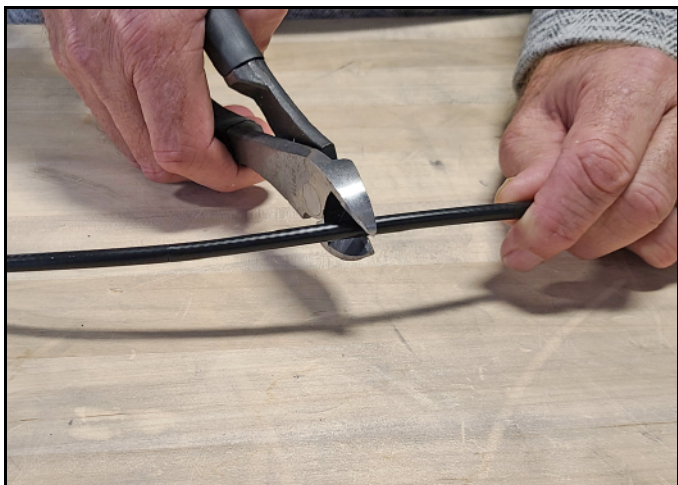
Figure 45: Cutting the Cable
