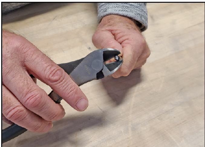
Figure 46: Reshaping the Cable
