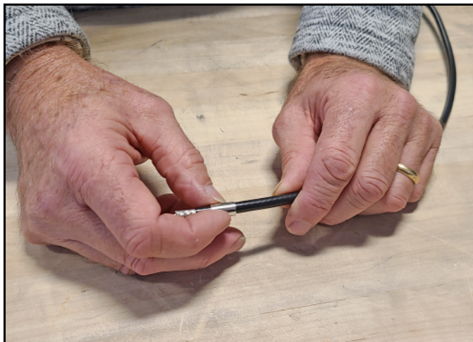
Figure 47: Placing the Ferrule
