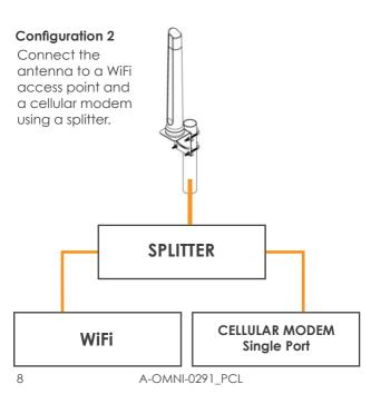
\* When mounting two OMNI 291 antennas in a LTE configuration: Space the antennas as far apart as possible, with a minimum distance of 1.5m
