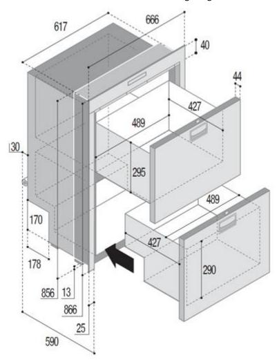
Built-in dimension with Door Inside - Door Outside mounting flanges
