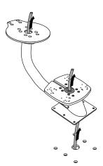
Lower the mount **16** onto the mounting platform. Be sure to line up the mount with the six bolt holes you previously drilled.
