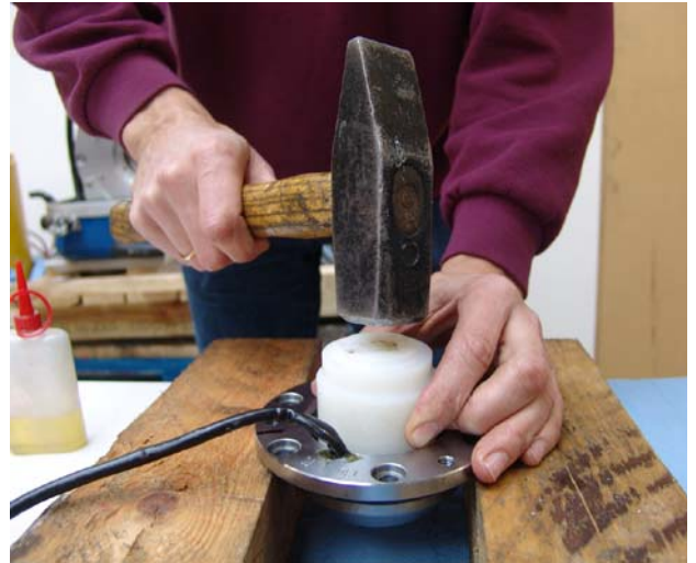
Fig. 7.12.2-17: Fitting the shaft sealing ring
