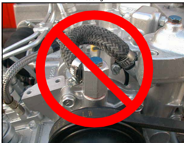
Fig. 7.14-5: Ventilation screw above the cooling water pump casing
