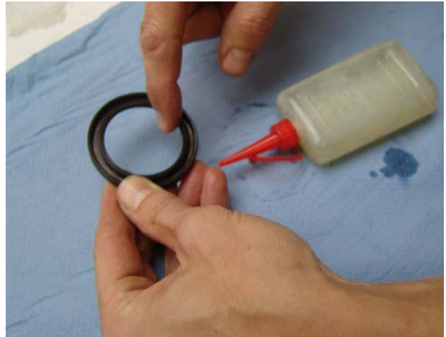
Fig. 7.12.2-14: Mounting the shaft sealing ring
