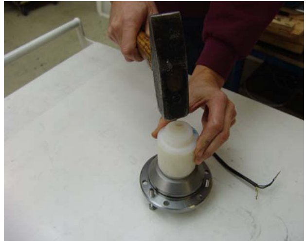
Fig. 7.12.2-11: Dismounted shaft sealing ring
