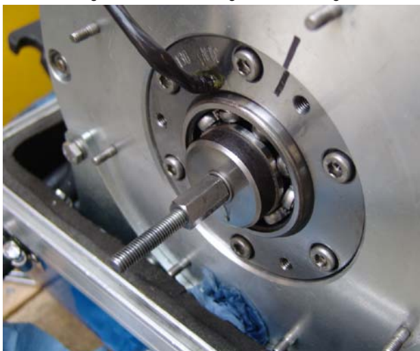
Fig. 7.12.2-27: Mounting the ball bearing
