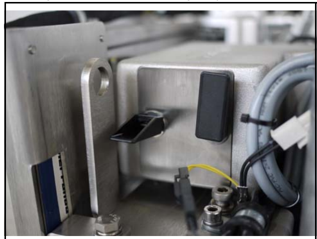
Fig. 7.14.2-3: Air suction housing with pull out holder
