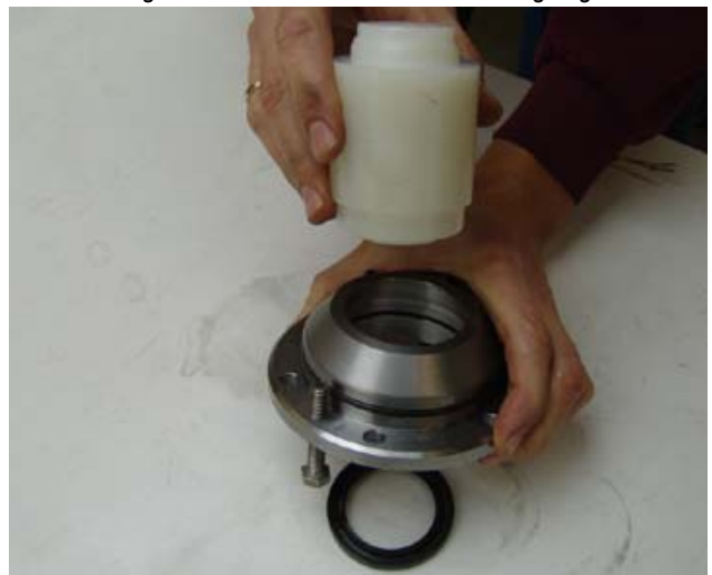
Fig. 7.12.2-11: Dismounted shaft sealing ring
