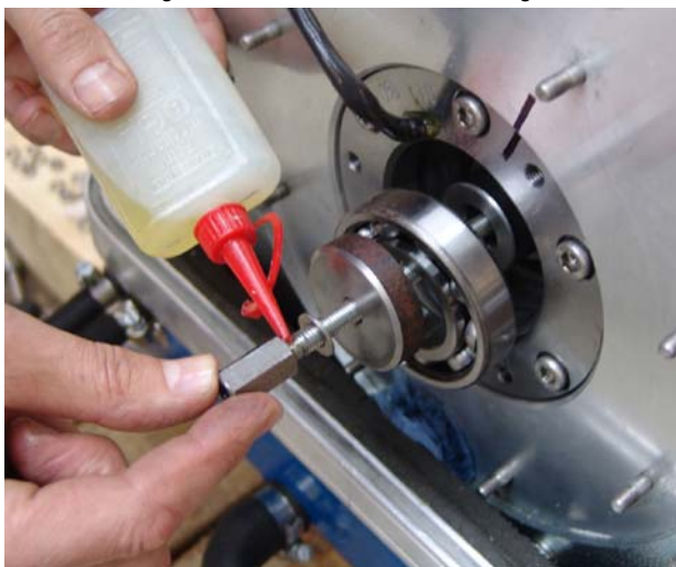
Fig. 7.12.2-26: Mount the ball bearing
