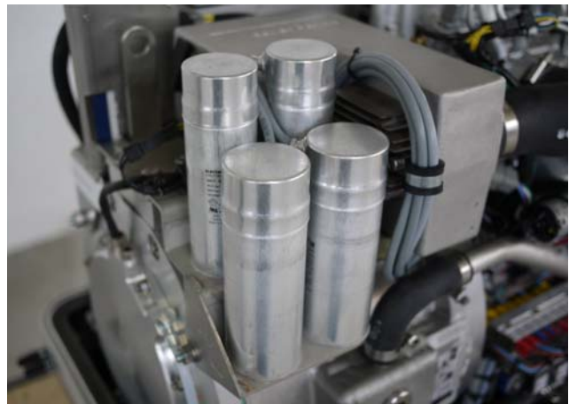
Fig. 6.11.4.1-2: Capacitors at the Panda 6000 ND PMS
