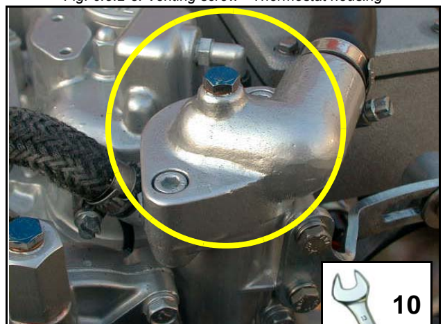
Fig. 6.5.2-3: Venting screw - Thermostat housing
