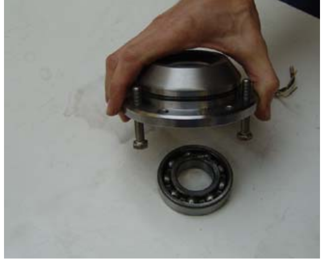
Fig. 7.12.2-10: Dismount the shaft sealing ring
