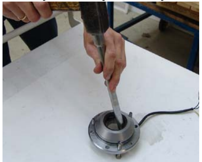
Fig. 7.12.2-8: Knocking out the ball bearing
