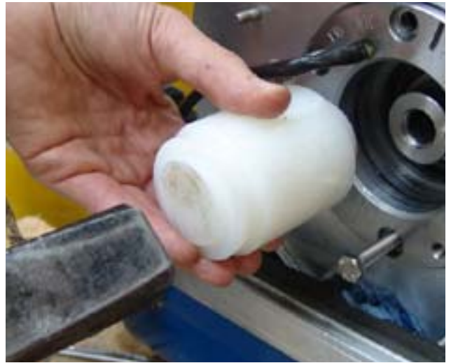
Fig. 7.12.2-23: Mount the bearing housing
