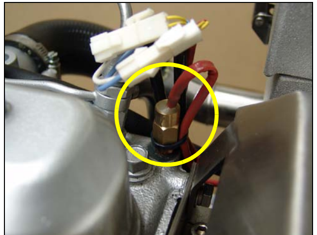
Fig. 4.3.5-1: Thermo-switch at cylinder head
