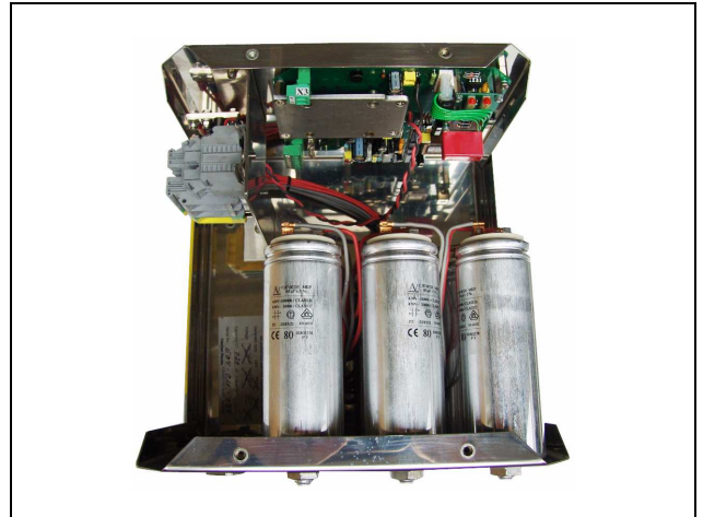
Fig. 4.3.7-2: AC Control Box - Opened
