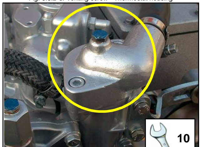
Fig. 5.5.2-3: Venting screw - Thermostat housing
