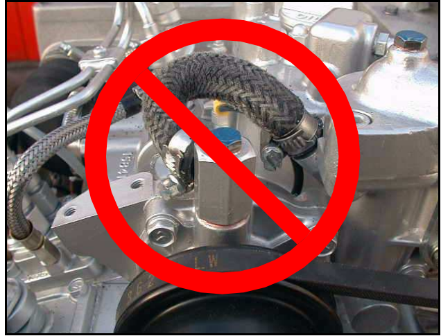
Fig. 6.12.0-5: Ventilation Screw above the Cooling Water Pump Casing
