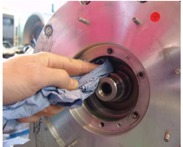
Fig. 6.10.2-19: Cleaning the shaft
