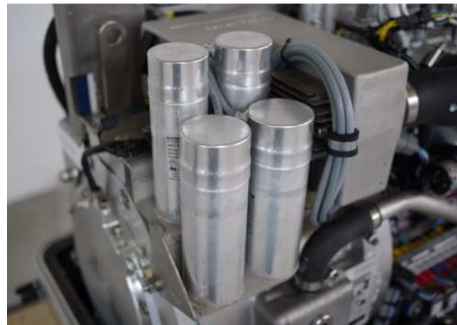
Fig. 5.10.4.1-2: Capacitors at the Panda 6000 ND PMS
