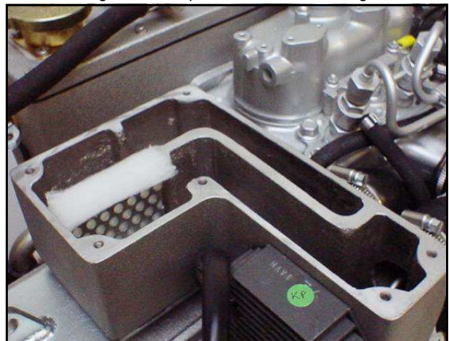
Fig. 6.11.3-2: Opened Air Suction Housing
