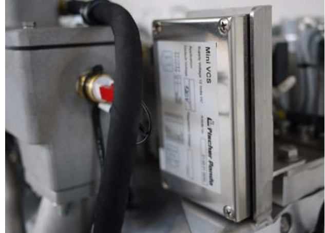
Fig. 5.10.4.1-2: Capacitors at the Panda 6000 ND PMS
