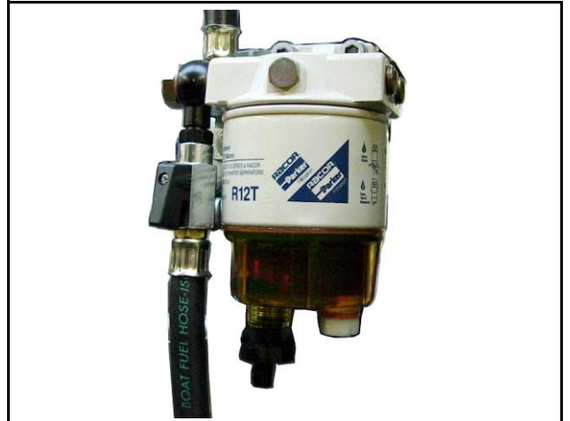
Fig. 6.12.1-1: Fuel filter with water separator
