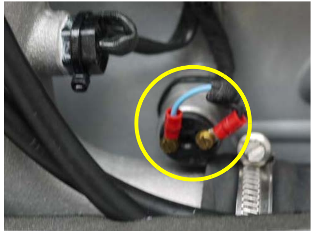
Fig. 4.3.5-4: Oil pressure switch
