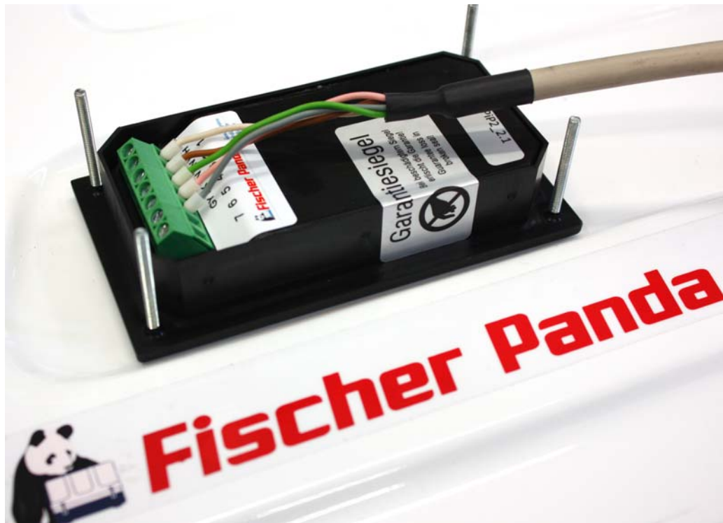
Fig. 3.2.1-1: Panda iControl2 panel with panel connecting cable and closed housing
