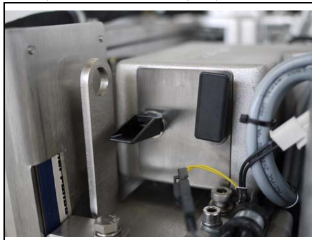
Fig. 7.14.2-3: Air suction housing with pull out holder
