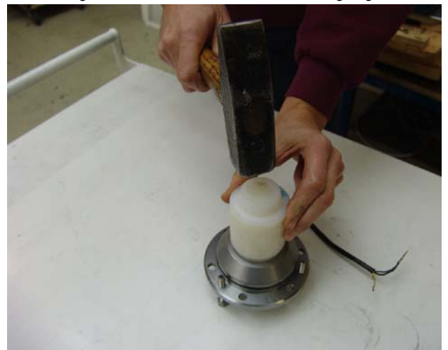
Fig. 7.12.2-11: Dismounted shaft sealing ring
