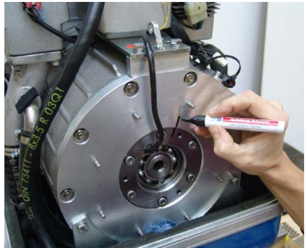
Fig. 7.12.2-5: Loosen fastening screws
