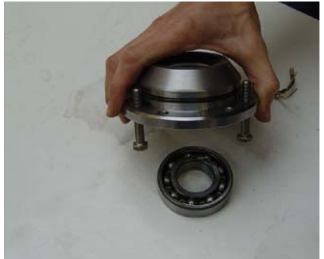
Fig. 7.12.2-10: Dismount the shaft sealing ring
