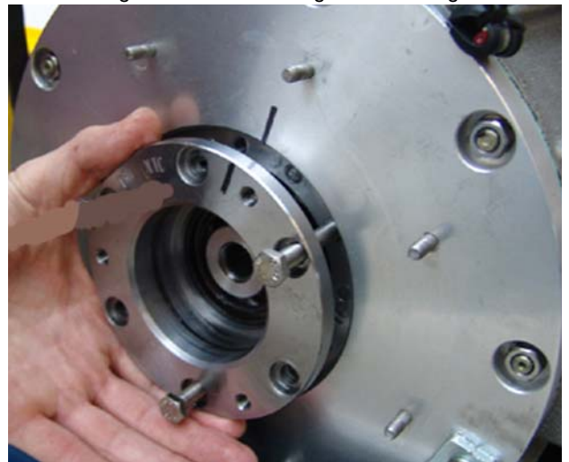
Fig. 7.10.1.3-2: Bearing case mouting
