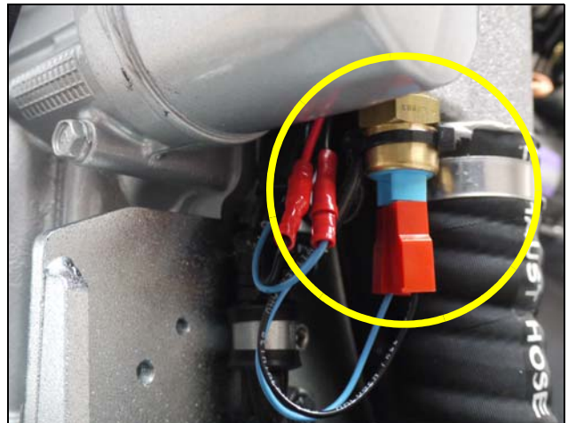
Fig. 4.3.4-2: Thermo-switch at exhaust connection
