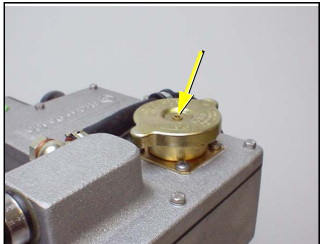
Fig. 7.14-4: Cooling water filler cap
