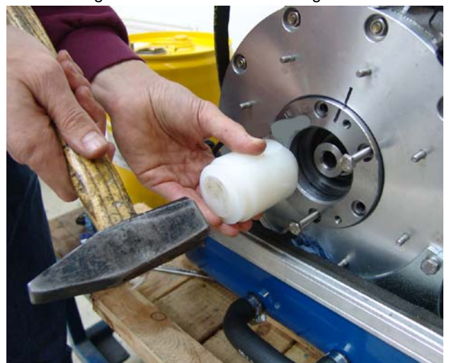
Fig. 7.10.1.3-3: Press fit bearing case
