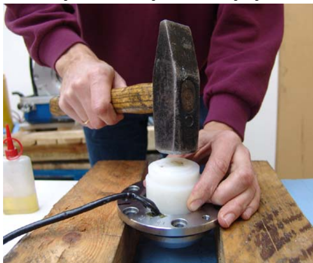
Fig. 7.12.2-17: Fitting the shaft sealing ring
