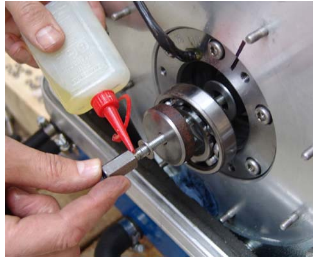
Fig. 7.12.2-27: Mounting the ball bearing
