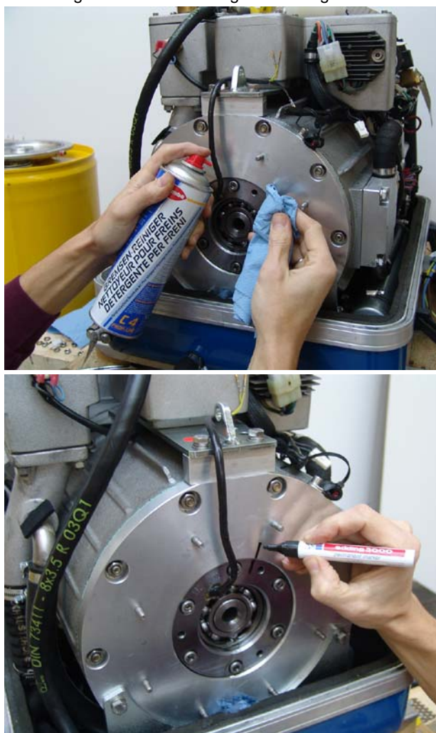
Fig. 7.10.1.2-1: Marking the bearing cover.
