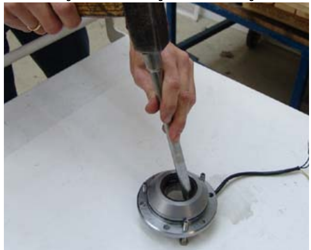
Fig. 7.12.2-8: Knocking out the ball bearing
