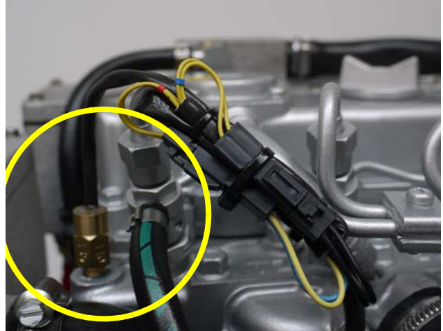
Fig. 4.3.4-1: Thermo-switch at cylinder head
