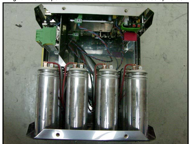
Fig. 6.11.3-2: Opened AC Control Box from Panda 30 upwards
