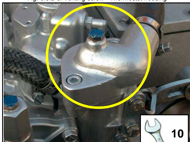
Fig. 6.5.2-3: Venting screw - Thermostat housing
