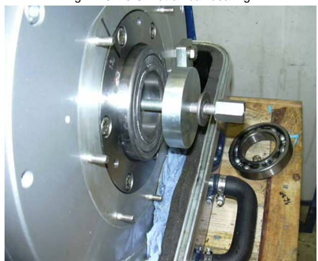
Fig. 7.10.1.3-6: Put on ball bearing
