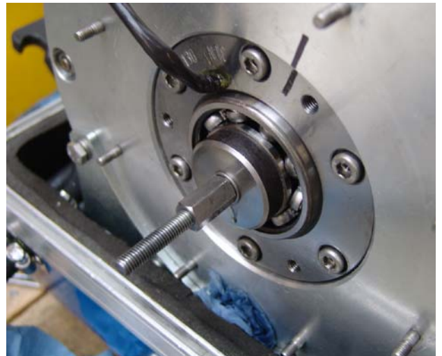
Fig. 7.12.2-28: Mount the ball bearing
