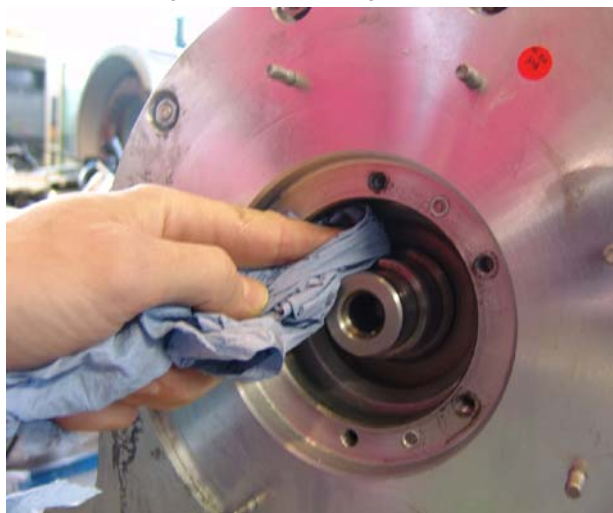
Fig. 7.12.2-19: Cleaning the shaft
