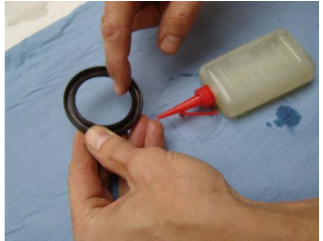
Fig. 6.12.2-14: Mounting the shaft sealing ring
