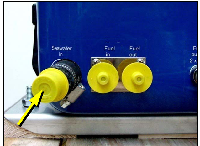
Fig. 4.3.1-1: Raw water intake
