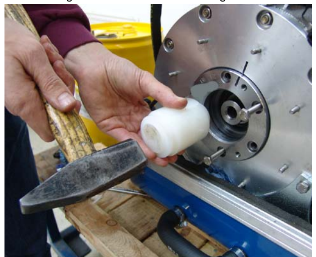
Fig. 6.10.1.3-3: Press fit bearing case
