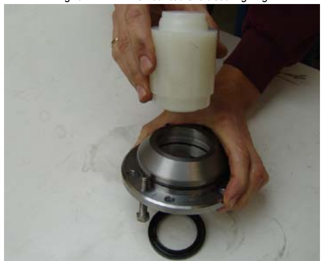
Fig. 6.12.2-11: Dismounted shaft sealing ring
