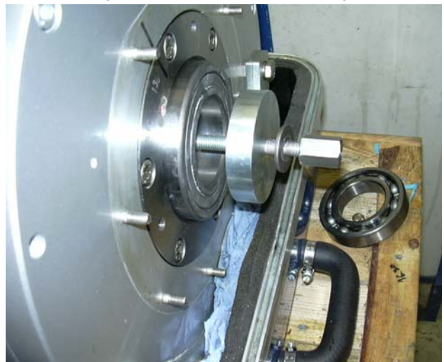
Fig. 6.10.1.3-6: Put on ball bearing
