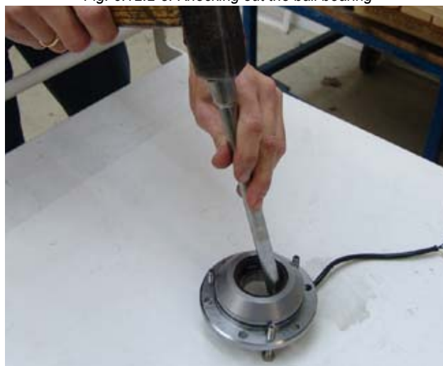
Fig. 6.12.2-8: Knocking out the ball bearing
