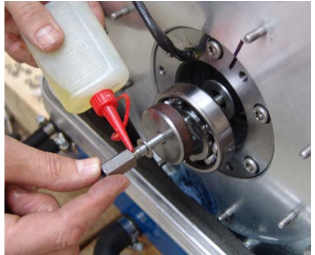
Fig. 6.12.2-27: Mounting the ball bearing
