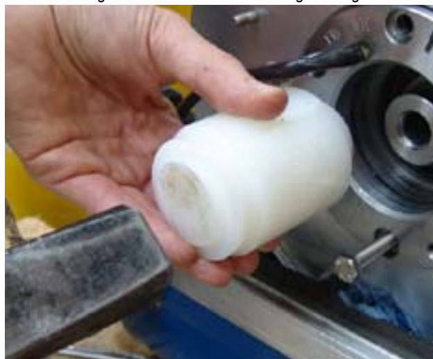
Fig. 6.12.2-23: Mount the bearing housing
