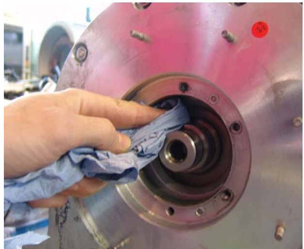
Fig. 6.12.2-19: Cleaning the shaft
