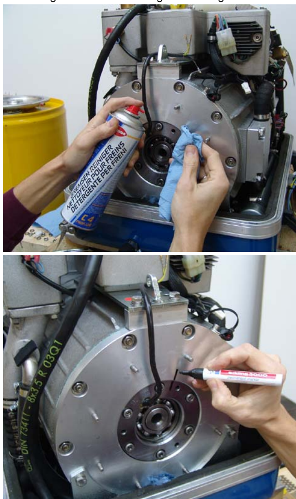
Fig. 6.10.1.2-1: Marking the bearing cover.
