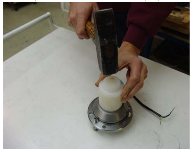
Fig. 6.12.2-11: Dismounted shaft sealing ring
