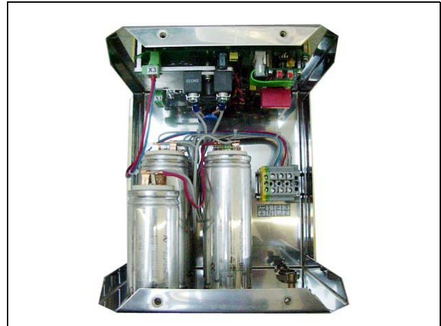
Fig. 4.3.8-2: Opened AC-Control box
