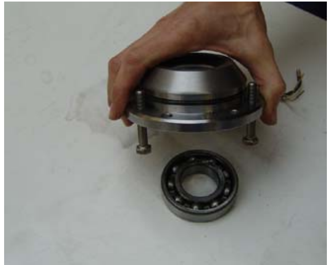
Fig. 6.12.2-10: Dismount the shaft sealing ring
