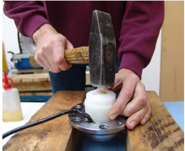
Fig. 6.12.2-17: Fitting the shaft sealing ring
