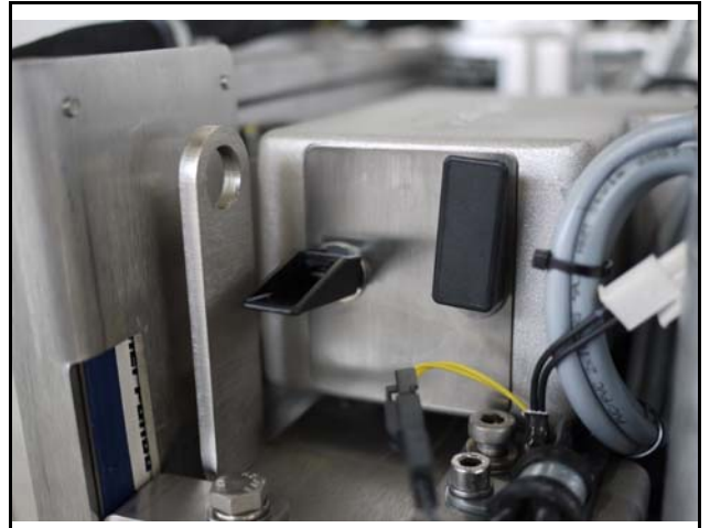
Fig. 6.14.2-2: Air suction housing with pull out holder
