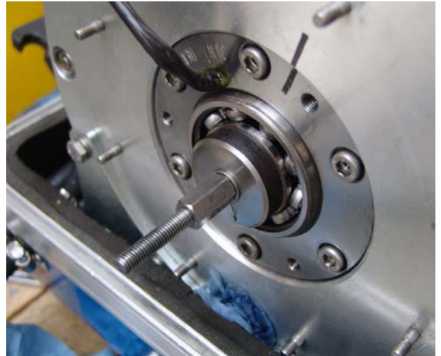
Fig. 6.12.2-28: Mount the ball bearing
