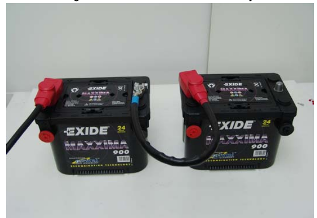
Fig. 5.12.2-3: Installation starter battery
