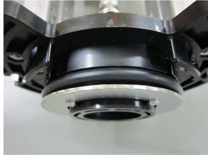
Insert the rubber bush into transducer part.
