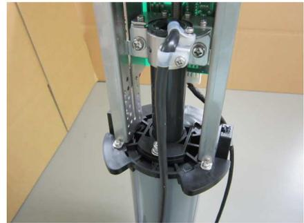
PCB side has the connection between power and Upper/Lower signal lines. The opposite side has the transducer cable.
