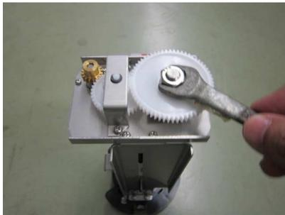
Caution: Do NOT raise the soundome too high. That causes the damage onto the upper limit switch. Raise the soundome by looking at the positioning of limit switch and operation lever.
