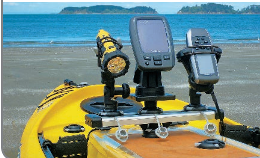
03-4102-11 TracPort Dash 500 Includes 500mm (19.5 in) Track with 4 StarPorts installed and 2 attachment adaptors
